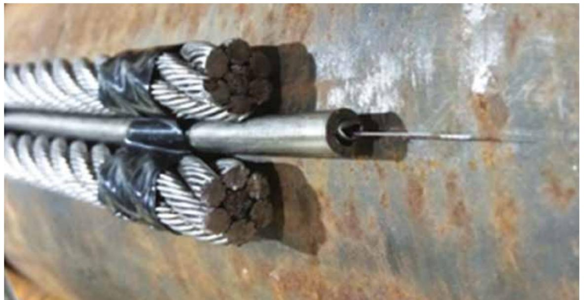
An example of a fibre-optic cable configuration which is used for DAS. Within the above cable, there are four strands illustrated – two single mode fibres and two multimode fibres.
