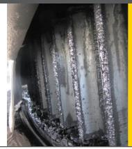
Poor adhesiveness results in unprotected open gear tooth surfaces. **Competitor's** product on electric shovel at same site
