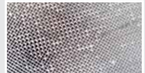
RIGHT: Similar section from engine using ~1% ash oil, such as Shell ROTELLA® T4 Triple Protection showing less blockage (fewer white areas.)
